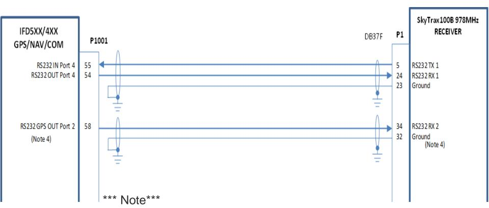
The ST100B only needs to be connected to a single IFD in multiple IFD installations. All of this data will cross-sync to the opposite IFD.
