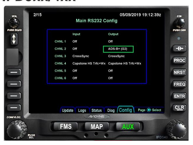
ADSB+(G2) to provide GPS data to the ST100B at 38,400 Baud Rate
