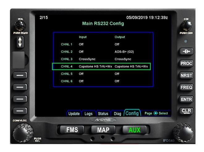
Capstone HS Trfc & Wx to and from the ST100B for ADSB traffic and FIS B weather Display at 115,200 Baud Rate
