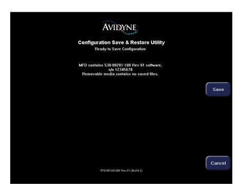
4. \_\_\_\_\_ Press "Save" to proceed with saving the configuration data to disk, or "Cancel" to discontinue the operation and allow the MFD to boot normally.
