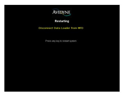
11. \_\_\_\_\_ Remove the CSR Utility USB flash drive from the MFD and press any bezel key.
