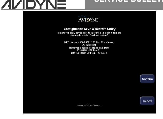
8. \_\_\_\_\_ Press "Confirm" to proceed with the Restore process, or "Cancel" to discontinue the operation.
