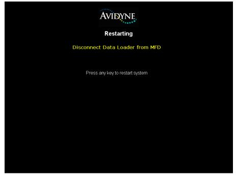
11. \_\_\_\_\_ Remove the CSR Utility USB flash drive from the MFD and press any bezel key to restart the system. After a few seconds the Maintenance Mode screen will appear as below (or similar):
