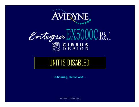
12. \_\_\_\_\_ Power down the MFD. The MFD can now be removed from the aircraft and the upgrade Compact Flash replaced.
