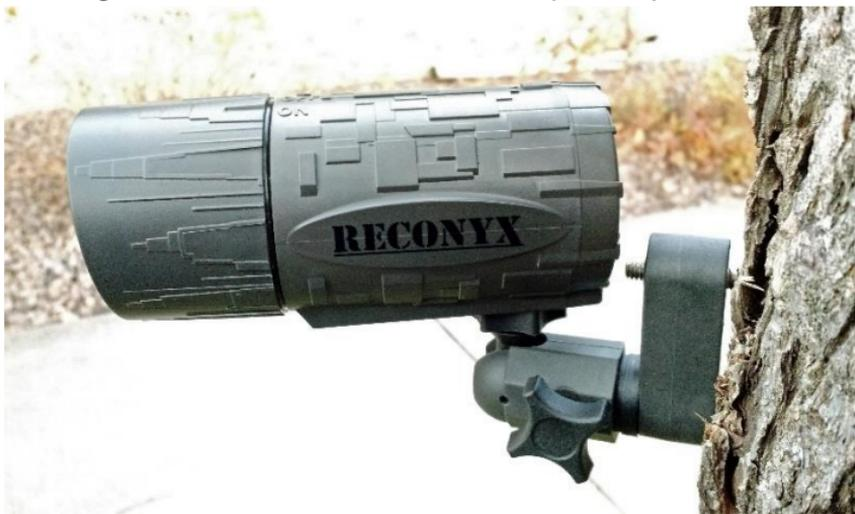
We recommend that you mount your camera at a height of approximately 4 feet or higher. This height is optimal for detecting animals in the field of view of the camera as well as for accessing the camera's card and batteries.
