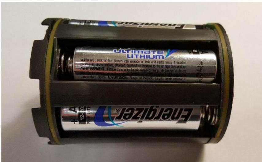
**Warning!** Do not mix battery types! Damage to the camera can result and your warranty will be voided if you mix battery types.
