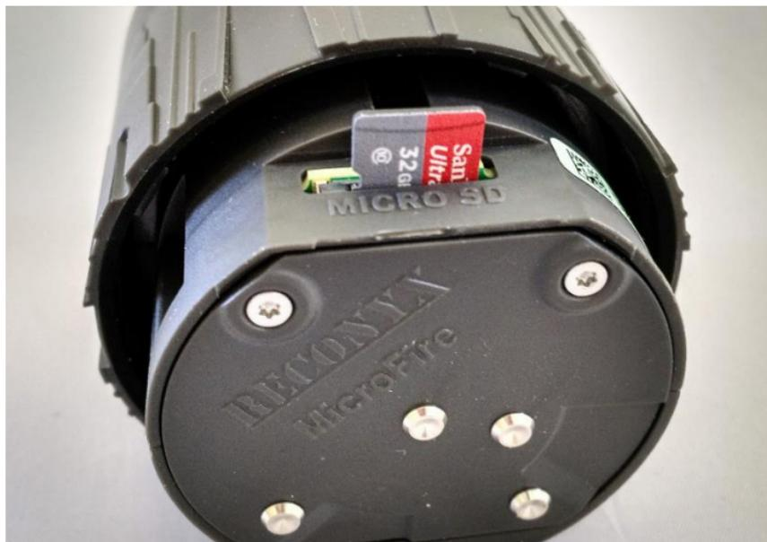
**Warning!** Inserting the memory card upside down or backwards could damage the camera or the memory card. Damage resulting from inserting the card incorrectly is not covered under warranty.
