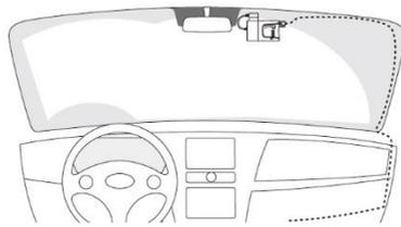
The cable supplied will allow you to hard wire the CP1 unit to the power source (i.e. fuse box) of your vehicle.
