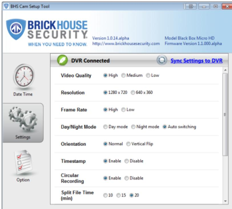
The BHS Cam Setup Tool is divided up into 3 sections. When the device is plugged into your PC via USB, the icon along the top will say “DVR Connected”. If it says “DVR Disconnected,” you may need to power your computer off and on and plug the device back in.
