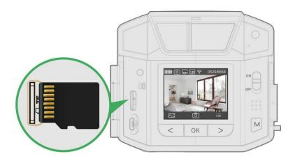
When inserting or removing the SD card, please make sure that the camera is turned off.
