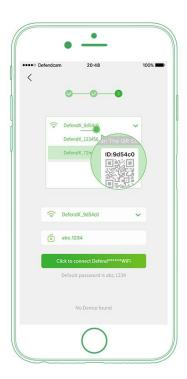
6.For Android users, please connect your camera Wi-Fi according to the ID on the QR code. Then it will prompt the boot operation after success or failure.
