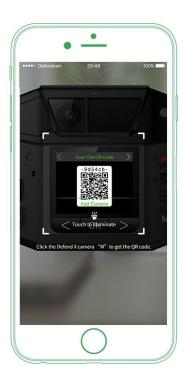
3.Switch ON camera, please press menu button to enter main interface. Scan QR code on the camera.
