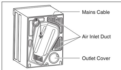
You can position the vent kit at the back of the dryer to remove air upwards or sideways.
