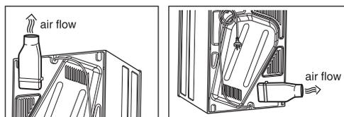
Inlet and outlet points need clear airflow to prevent overheating, so ensure there is adequate ventilation. (i.e. open window or external door.)
