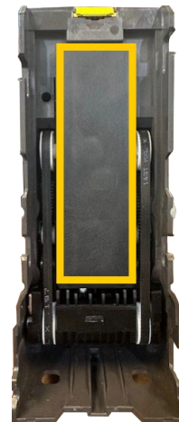
Fig. 7: The rear stacker plate
