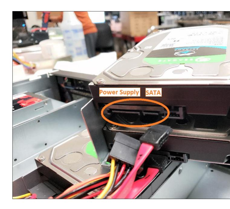
3) Remove the **four (4) mounting screws** that secure the HDD to the mounting bracket, then carefully **remove the HDD** from the mounting bracket.
