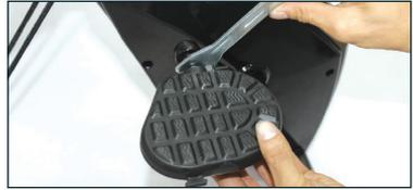
Hold the right pedal with one hand and screw the pedal bolt onto the crank arm with the other hand in a **standard clockwise** motion. Finish tightening with the included wrench.
