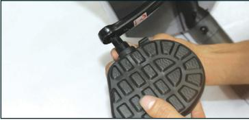
Connect the right pedal to the right crank arm. Both parts are marked **R**.
