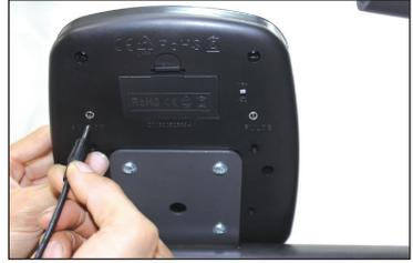
Connect heart rate wire to the control panel.
