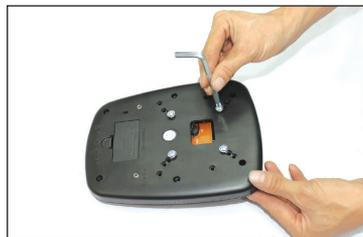
Remove screws from the back of the control panel.
