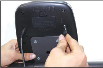
Connect the sensor wire with the L-shaped plug to the control panel.
