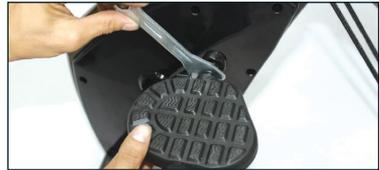
Hold the left pedal with one hand and screw the pedal bolt onto the crank arm with the other hand in a **non-standard counterclockwise** motion. Finish tightening with the included wrench.
