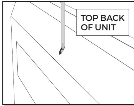
2. Using a Philips screwdriver, drive in the screw located above wall mount to secure.
