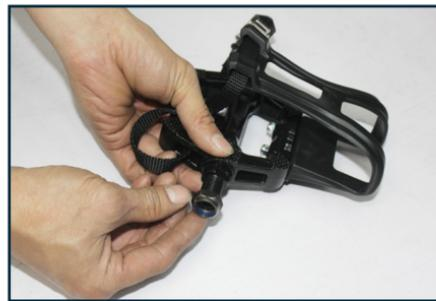
**The threads are reversed on LEFT pedal and nut.**
