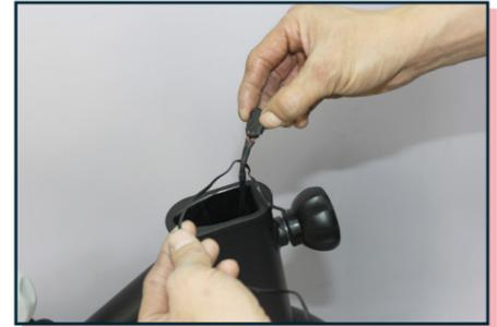
Pull out the wire, ensuring not to allow the wire to fall inside frame.
