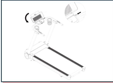
Press and hold the Tablet Adjustment Lever and then rotate Tablet holder backwards until flat with the handlebars.
