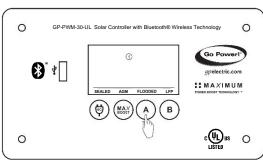
Next, select the charging profile of battery bank 1 by pressing the **B Button** to toggle through the profile options: Sealed/Gel, AGM, Flooded, or LFP. To confirm the battery profile, press and hold the **A Button** for 3 seconds.
