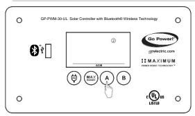
To select the charging profile of battery bank 2, press the **B Button** to toggle through the profile options: Sealed/Gel, AGM, Flooded, or LFP.
