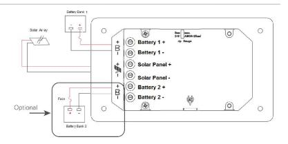
The fuses or breakers used should be no larger than 50 amps.
