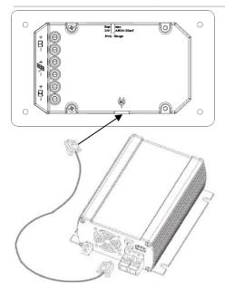
First, connect the inverter directly to the battery (follow the installation instructions included with the inverter).
