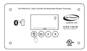
Now you can turn the connected inverter on or off by holding down the **AC Symbol Button** for 3 seconds.
