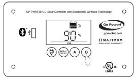
The battery state of charge is shown as a percentage. **Icons Displayed**: Battery SOC, Percent Symbol (%), Symbol 2
