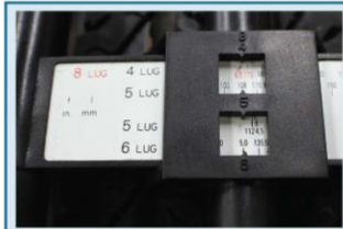
A six lug wheel has 5.0" lug spacing.
