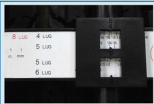
A four lug wheel has 108 mm lug spacing.
