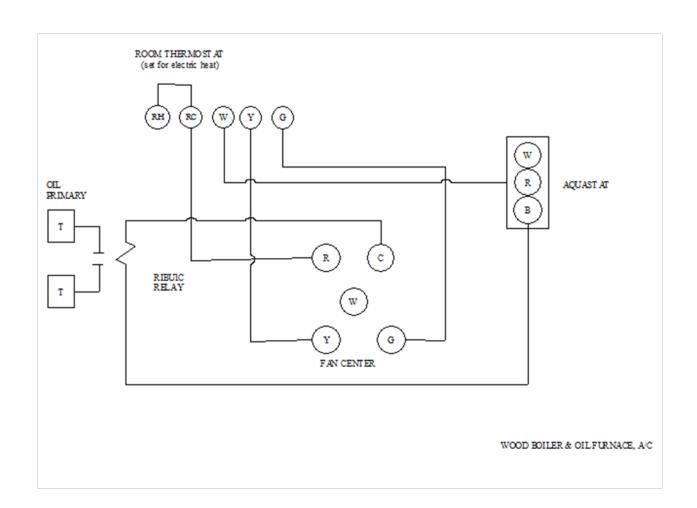
THIS SYSTEM INCLUDES A FORCED AIR ZONE PANEL WITH A FURNACE DIVERTING VALVE AND WOOD BOILER. WHEN A ZONE CALLS FOR HEAT THE PANEL SENDS A "W" SIGNAL TO THE AQUASTAT THAT DIRECTS IT TO THE DIVERTING VALVE IF THE BOILER IS WARM OR TO THE FURNACE IF THE BOILER IS COLD
