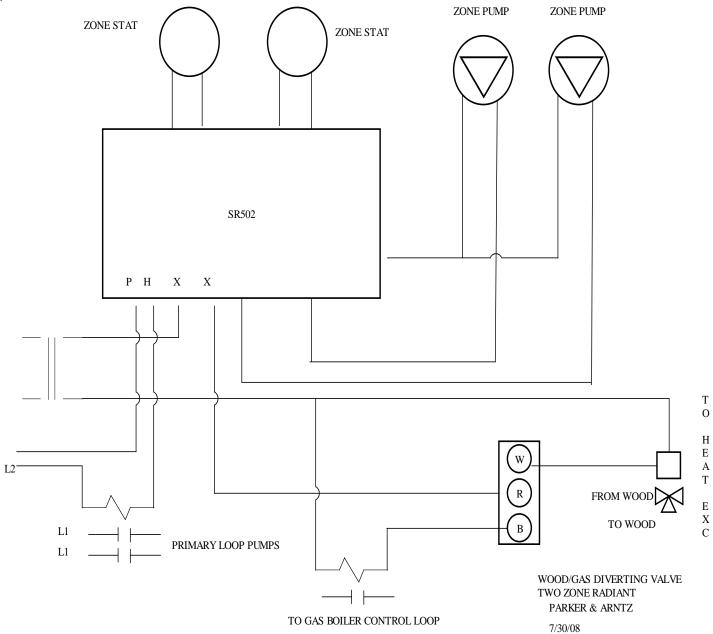
Wood Boiler, Air Source Heat Pump, and Propane Furnace under the control of a Honeywell IAQ thermostat: First call for heat can be either heat pump or boiler. The three way valve prevents heating of the boiler loop with the propane furnace if the second stage of heat calls or if the heatpump is in low temp lock out and the boiler has no heat available
