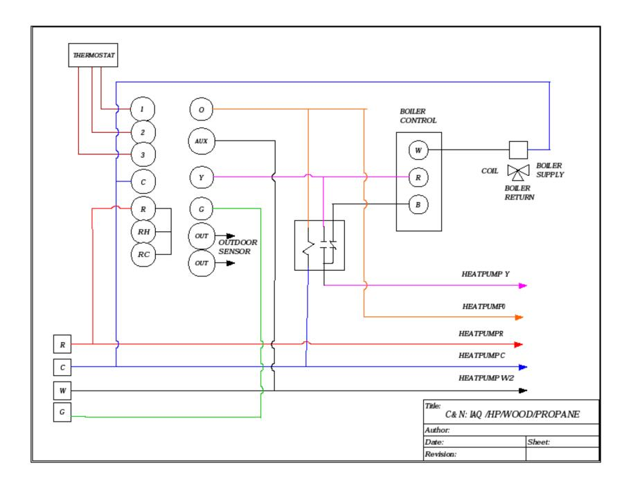
Some furnaces that have integrated fan controls need to run the high speed for the hot water coil but low speed for the furnace. This one takes care of the isolation of the fan signal for each condition.
