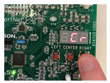
Then press "CENTER" to select the Cr menu. Some codes will begin flashing on the display. Ignore these codes and hold down the "LEFT" and "RIGHT" buttons simultaneously for at least
