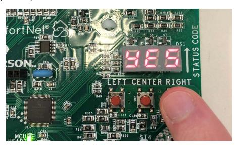
Then press the "CENTER" button **twice** to confirm the selection. The board will then start the Shared Data loading process. Once the Shared Data Loading process is complete, the display will return to displaying "Cr".
