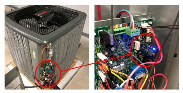
The reprogrammable Shared Data loader card must be powered on to load Shared Data onto a unit
