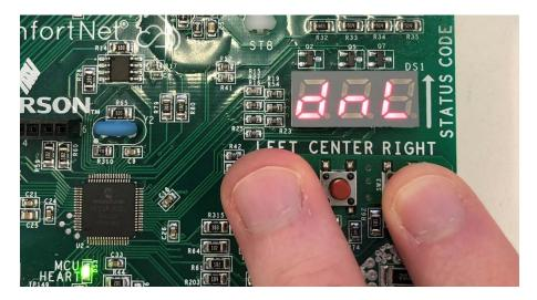
After holding "LEFT" and "RIGHT" for 10 seconds, the display will start flashing a new code ("dnL"), once this new code appears, release the "LEFT" and "RIGHT" buttons. The equipment will display the options "YES" and "no" to confirm or cancel the Shared Data loading process. To confirm the process, press the "RIGHT" button to select "YES".
