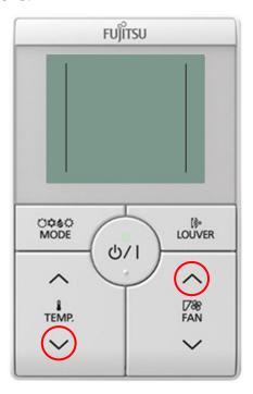
14. The Remote Control sensor icon should be displayed to confirm the function setting change from Steps 11 & 12.
