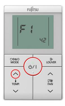
4. Access the Function Settings menu by using the TEMP up arrow, and scroll to item setting 13. When item setting 13 is flashing, press the START/STOP button to enter the Function Settings Menu:
