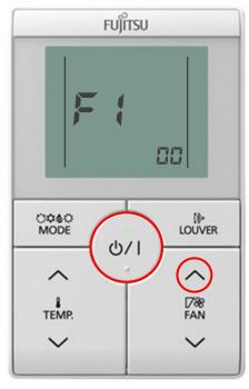
12. Use the TEMP up arrow to adjust setting option to 01. Press the START/STOP button to assign the
