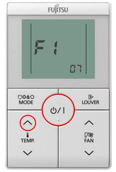
10. When A1 flashes, press and HOLD the FAN up arrow until F1 is displayed for the Initial Settings mode:
