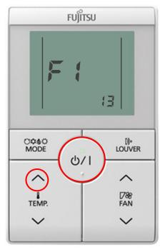
6. Use the TEMP up arrow to adjust the default setting option from 00 to 01. Press the START/STOP button to assign the setting option. Note: Remote controller address "002" does not need to be changed. Press the START/STOP button to proceed to function setting adjustment
