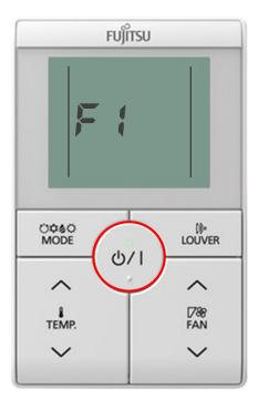
5. Use the TEMP up arrow to scroll to function setting 42. Press the START/STOP button to open the function setting option selection.
