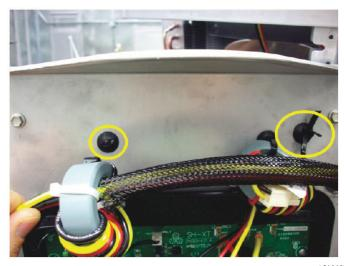
7. Remove top two screws holding control box and remove compressor harness (highlighted in yellow below).
