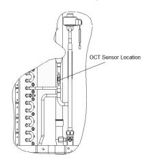
Fig. 3 - HP Outdoor Coil Thermistor (OCT) Attachment (On Distributor Tube)
