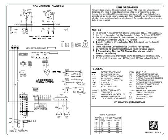
Fig. 37 - \*VA9 WIRING DIAGRAM - Sizes 25, 36, 37, 48, 49, 60
