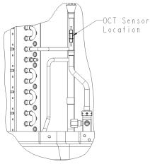
Fig. 4 - AC Outdoor Coil Thermistor (OCT) Attachment (On Distributor Tube)
