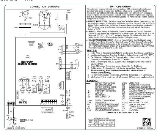
Fig. 38 - \*VH8 WIRING DIAGRAM - Size 24
