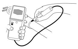
Fig. 43 - Electronic Leak Detection
