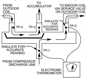
Fig. 41 – Reversing Valve (Heating Mode, Solenoid De-Energized)
