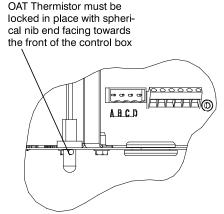
Fig. 2 – OAT Thermistor Location (Bottom of Control Box)
