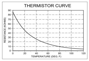
Fig. 29 – 10K Thermistor Resistance Vs Temperature
