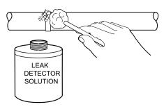
Fig. 44 - Bubble Leak Detection
