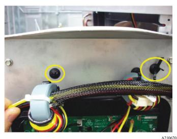
Remove top two screws holding control box and remove compressor harness (highlighted in yellow below).
