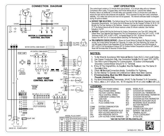
Fig. 39 - \*VH8 WIRING DIAGRAM - Sizes 25, 36, 37, 48, and 60
