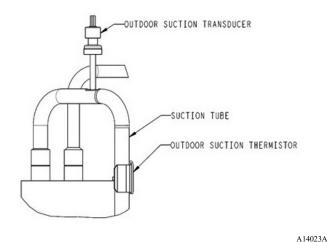
Fig. 5 – Suction Thermistor (OST) Attachment (On Suction Tube)
