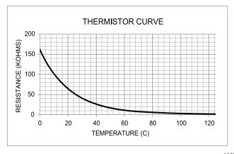
Fig. 30 – 50K Thermistor Resistance Vs Temperature
