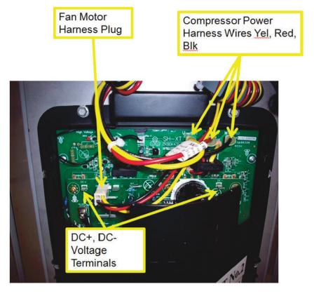
Fig. 32 – Compressor and Fan Harness (Unit sizes 25, 36, 37, 48, 49 and 60)
