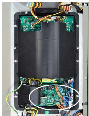
Fig. 1 – AOC (Application Operational Control) Board
