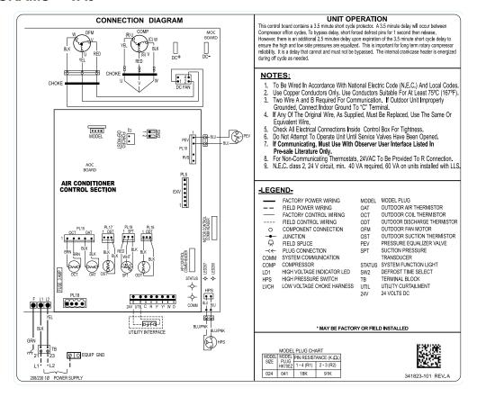
Fig. 36 - \*VA9 WIRING DIAGRAM - Size 24
