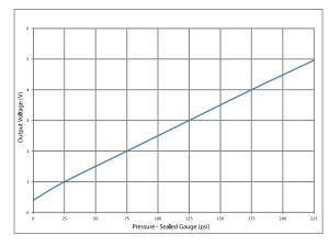
Fig. 28 – Suction Pressure Transducer (SPT)
