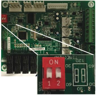
Fig. 7 - AOC Control Board for 1 and 2 Ton
