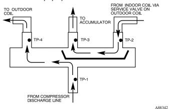
Fig. 40 – eversing Valve (Cooling Mode or Defrost Mode, Solenoid Energized)
