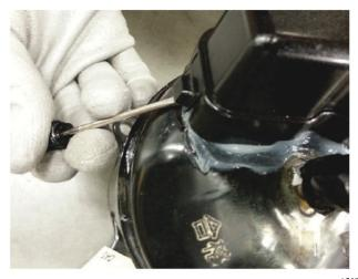
A210662 10. It may be necessary to leverage the screwdriver against cover next to tab so as not to break the tab while loosening.
