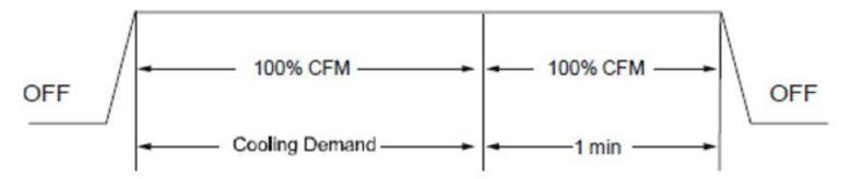
Profile B(2) ramps up to full cooling demand airflow by first stepping up to 50% of the full demand for 30 seconds. The motor then ramps to 100% of the required airflow. A one (1) minute OFF delay at 100% of the cooling airflow is provided.
