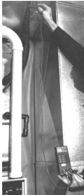
FIGURE 49 TEMPERATURE RISE MEASUREMENT
