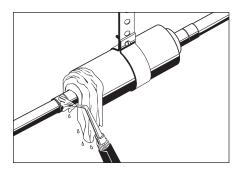
All sealed model suction line filters and filterdriers have copper fittings. It is not necessary to clean the fittings prior to brazing.
