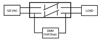
Load example: 600-Watt heater (600 W = 600 VA - 120V x 5A)
