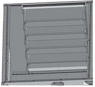
Next re-install the parts removed in step 3 into new parts added parts 0121L05291 (left) and 0121L05292 (right). There are new sets of holes to screw these parts into. Please note, the bottom filter support will also need to be screwed into 0121L05244 as well.
