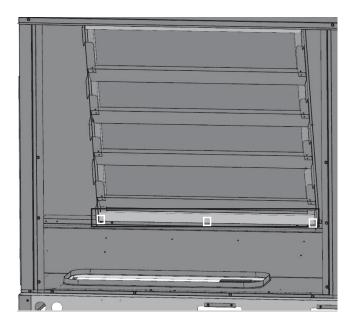
8. Next install the new 0121L05242 top block off where the old top block off was removed in step 2b.
