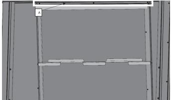
3. Begin by removing the [1] Top Filter Support, [2] Middle Support, and [3] Bottom Support. Keep the screws and make note of the locations, as we will install the next parts in these same holes.
