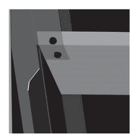
6. Next install the [2] bottom louver 0121L05294. This will use 5 screws total, 4 on the sides just as seen in step 5 and one where the additional hole is for the flashing kit. This bottom louver will be inserted between the [1] filter rack and the [3] evaporator coil as seen in the second image.(Various panels were hidden for clarity purposes).
