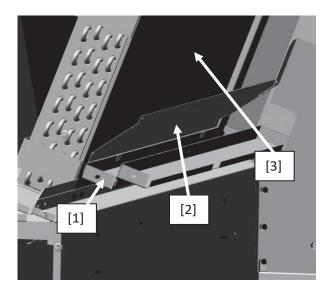
7. Next install the 0121L05244 bottom block-off where the bottom filter rack part used to be. Use the large clearance holes to insert the back screws (seen in boxes below)
