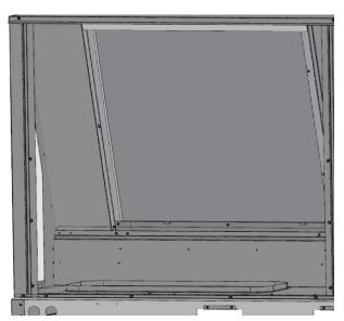
4. Next Install parts 0121L05291 (left) and 0121L05292 (right) on the left and right sides of the filter rack as seen below. They use the same holes which the old filter rack parts previously used.
