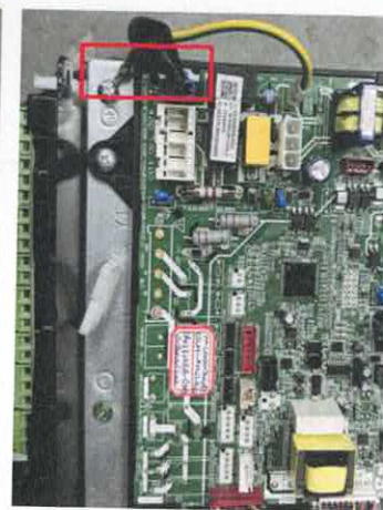
CN12 port on main control board
