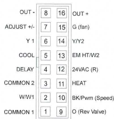
CONTROL CONNECTOR "Motor Half" (Viewed from connector end)
