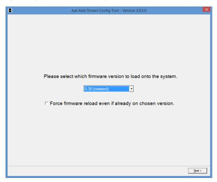
If you prefer to keep the currently installed version, choose "Don't Update Firmware" (note that this option won't appear if your connected JAP devices have mismatched firmware versions). If you want to re-install the same firmware version currently installed, check the box labelled "Force firmware reload even if already on chosen version".
