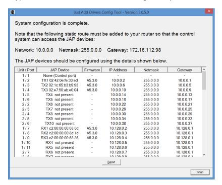
In addition, it also details the information required to set up the "static route" (consisting of a **Network** address, **Netmask** and **Gateway**). Be sure to note these down. A text file detailing the configuration is automatically saved in the installation directory (for example, *C: |Program Files (x86)|Just Add Power|JADConfig|Reports*) or can be generated by clicking **Export**.
