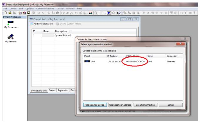
Note down the MAC address as highlighted above and send it to drivers@justaddpower.com in order to obtain your key. Note that if you do not obtain a licence key, the driver will operate in demonstration mode, allowing a maximum of 3 receivers and 3 transmitters (the driver will allow you to assign more than three ports, but only the first three will function).
