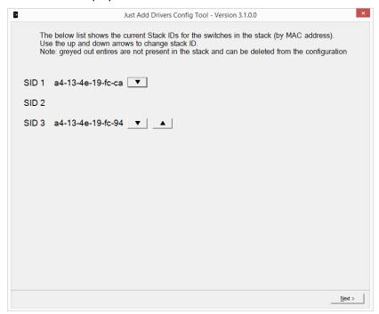
This screen identifies switches in the stack by MAC address. Use the **Up** and **Down** arrow buttons to change the Stack IDs of the switches in the stack. If a switch is no longer connected to the stack, its entry in the list will appear greyed out. Either reconnect it, or click on the **Delete** button to remove it from the configuration.
