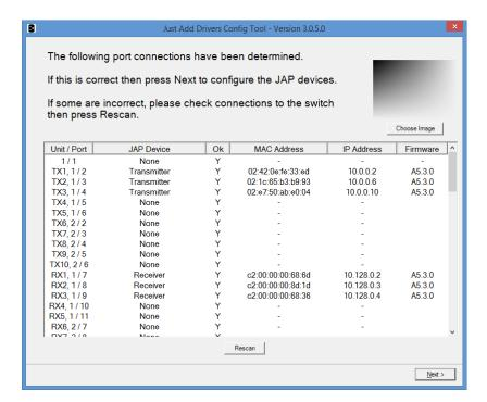
If some of your devices do not appear in the list of discovered devices, check the connections and press **Rescan**. In the event of errors, correct the patching as instructed. If you see a question mark displayed in the **Firmware** field, this may be due to duplicate IP addresses on two or more JAP devices. In this scenario, proceed with the configuration as the tool will resolve any such conflicts.
