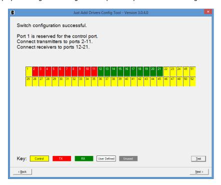
Note the **Test** button. This can be used to access a Test harness allowing you to test the switching functionality of your system. Refer to the section of this guide titled *Testing your System* for more information.
