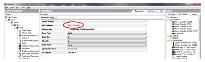
Note down this address and send it to drivers@justaddpower.com in order to obtain your key. Note that if you do not obtain a licence key, the driver will operate in demonstration mode, allowing a maximum of 30 minutes use before a driver reload is required.
