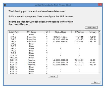
If some of your devices do not appear in the list of discovered devices, check the connections and press **Rescan**. In the event of errors, correct the patching as instructed. If you see a question mark displayed in the **Firmware** field, this may be due to duplicate IP addresses on two or more JAP devices. In this scenario, proceed with the configuration as the tool will resolve any such conflicts.
