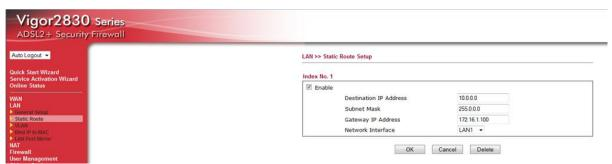
Enter the static route information from the final screen of the Just Add Drivers application into the **Destination IP Address**, **Subnet Mask** and **Gateway IP Address** fields.
