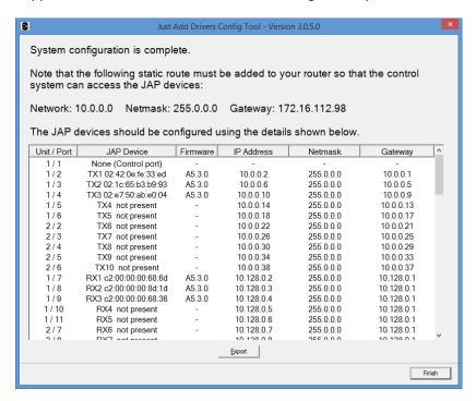
In addition, it also details the information required to set up the "static route" (consisting of a **Network** address, **Netmask** and **Gateway**). Be sure to note these down. A text file detailing the configuration is automatically saved in the installation directory (for example, *C: |Program Files (x86)|Just Add Power|JADConfig|Reports*) or can be generated by clicking **Export**.
