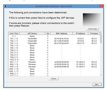
If some of your devices do not appear in the list of discovered devices, check the connections and press **Rescan**. In the event of errors, correct the patching as instructed. If you see a question mark displayed in the **Firmware** field, this may be due to duplicate IP addresses on two or more JAP devices. In this scenario,
