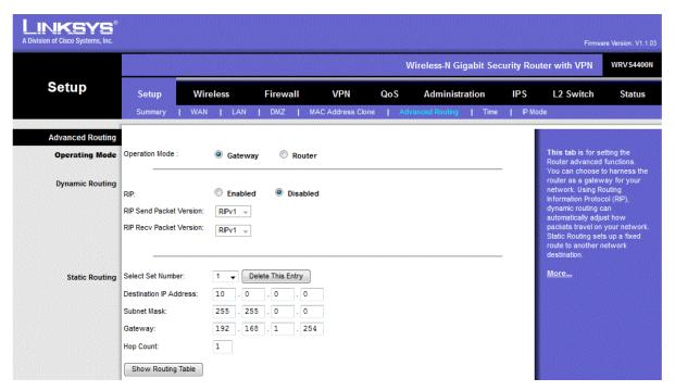
Enter the static route information from the final screen of the Just Add Drivers application into the **Destination IP Address**, **Subnet Mask** and **Gateway** fields.
