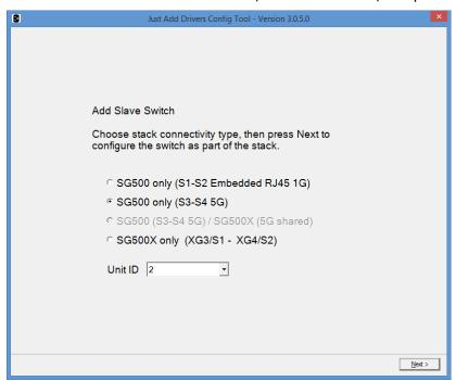
Choose the appropriate option depending on your Cisco switch model type and connection port. Next, select a **Unit ID** for the Slave switch.
