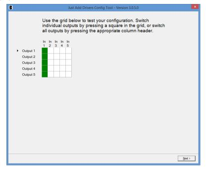
The application will automatically generate a test grid for your configuration. You can switch individual outputs by clicking on a square in the gird (green squares denote the current selection for each output), or switch all outputs by clicking the appropriate column header.
