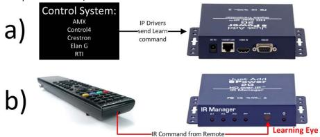
4. Program control system to send IR codes. Select bank, command, and "Emit" for code to be sent. When command is sent, the Activity Indicator Light will blink rapidly.
