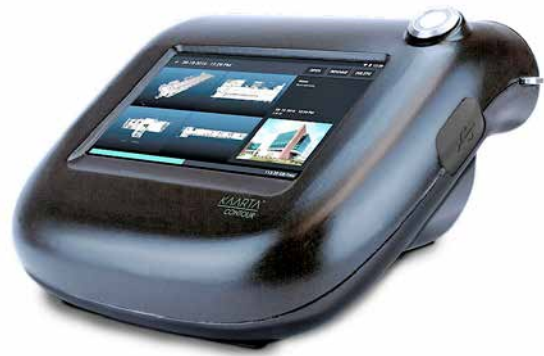
Figure 31 Kaarta Contour handheld laser scanner © Kaarta Inc
