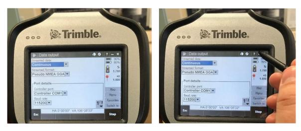
17) Make sure that the appropriate prism is selected by clicking the "red ball on a stick" icon (reflector-less measurements) and change it to the prism.
