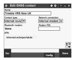
Clicking on the arrow from the Network connection will give you a list to choose from. Select Wi-Fi, ActiveSync and accept, then store the GNSS contact.
