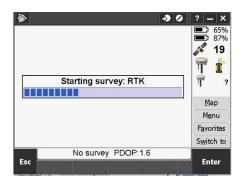
To start the Rover RTK survey, press Start survey and select the RTK & Infill option; this will initiate the radio connection to the Base. Wait for Radio Link icon to appear on the RHS display – this means that an RTK radio connection has been established between the Base and Rover. If prompted confirm <Accept> the Base station Index id.
