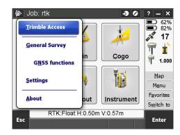
Use the various icons on the RHS of the screen to check battery levels, satellite positions, numbers being tracked and status.
