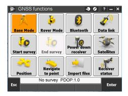
Then press Start Survey and select the survey style RTK. Follow the Start Base receiver steps.
