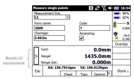
Clicking the **Esc** soft key cancels the current measurement and brings up the configuration panel again. Clicking the **Store** soft key stores the point and brings up the configuration panel again. If the measurement mode is set to "tracking" the result panel will still be displayed and the next point can be stored right away. The cursor will in both cases automatically jump back to the code field.
