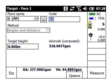
If the stationing type is "on a known point" the **Residuals dialog** will come up automatically after the first successful measurement. If the stationing type is set to "free stationing", an additional reference point has to be measured before the residuals dialog is displayed.
