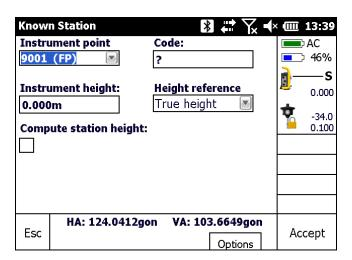
In the Options dialog the user may select if the station should be calculated with or without a scale. If you select without scale, the scale is set to 1.000000 automatically.
