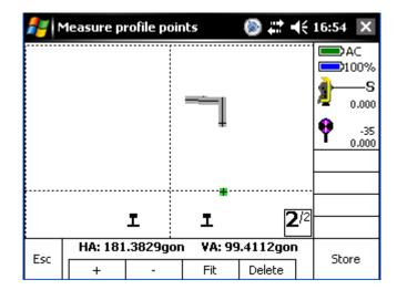
**Delete** will remove all selected points permanently. The **Store** soft key stores all new (green) points. If only a single point has been measured, the point is stored in the project's job file. If a scan has been performed, the points are stored in a separate file named after the current chainage (KM123+456.789) with the ending \*.scn. All files are stored in the subdirectory \Scans in the current project directory.
