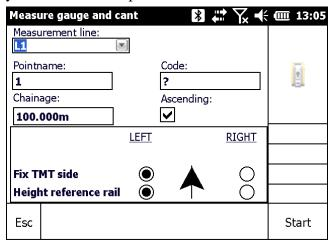
At beginning of measurement a line has to be defined. Settings for fixed trolley side and height reference rail have to be done as usual. Also specifying a chainage value for start point is recommended. Odometer implemented in wheel of movable trolley side is used for counting station values increasing or decreasing. The distance is measured on one rail so that there could be a difference between counted and real chainage especially in curves.
