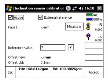
By pressing the soft key *Measure* the current sensor value is read out including the currently valid calibration and presented as current value. The default value, for example the value determined by a track rod will be entered in the provided field and therefore the new offset is calculated. *Accept* saves the new offset into the corresponding configuration file.
