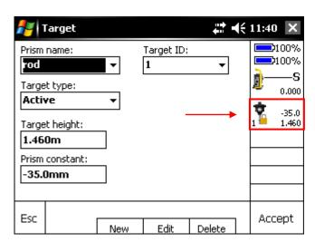
By clicking the "New" soft key a new prism definition can be added to the list. The name must not be equal to an already existing prism.
