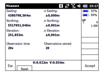
Option dialogue in continous measurement doesn't support the mean value. Instead the distance of auto storage can be defined like in total station measurement. Tracking mode will be started automatically when starting the contious measurement.
