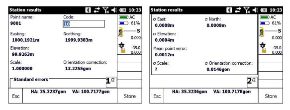
This now displays the results of the stationing, coordinates, orientation correction and the scale. On page 2 you can see the standard deviations for the calculated values. The mean point error is displayed as well.
