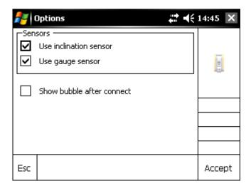
Additionally, if the respective box is checked the electronic level will be displayed after the connection to a total station is established successfully.
