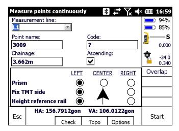
The **Start** soft key starts the measurement. The points are stored as soon as the given intervals are reached or passed. The result display is shown. The measurement line can no longer be edited in this mode. If a point should be stored although it does not fit the grid the user can press the **Store** soft key to store a point off the grid
