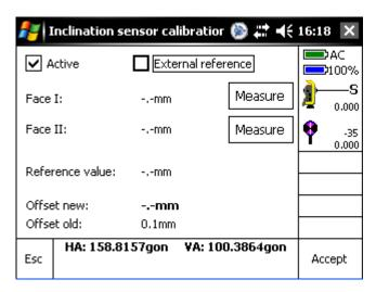
Note: If no sensor value can be received, this may have several reasons: The sensors get no or insufficient power (check the batteries, turn on the box), the wrong serial port is selected or the port parameters are wrong, the Bluetooth connection has a poor reception or is not setup correctly (terminate program, check settings of the operating system).
