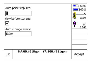
The textbox "**Auto storage every**" sets the step size after which in cases of a continuous survey the point is stored automatically. The minimum value is 0.1 meters. Using the "single survey" method the auto storage textbox will not be visible.
