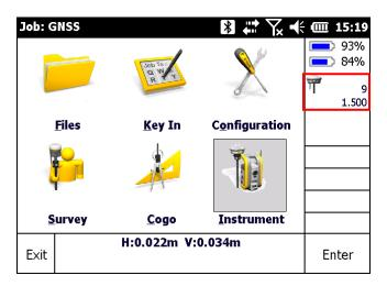
By clicking this field with antenna symbol, the dialog for receiver settings will open analogue to chap. 12.2. The antenna type and the length of the pole that were selected in Trimble Access can be seen and the user may enter an additional height offset. The final pole length will result as the summation of both offsets.
