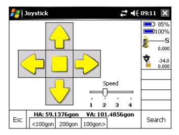
With the help of the soft keys below it is possible to turn the telescope by 100gon to the left or to the right or by 200gon.
