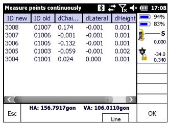
Last measurement line with identical line name will be used automatically for overlapping line. Line dialogue is displayed if a same-named line is not measured until now to select any other line. Use soft key Line to select a different line for comparison with the stations name, line name and timestamp (station setup time).
