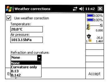
Additionally, measured values can be corrected by effects caused by refraction and earth curvature. Two models with the coefficients 0.13 or 0.142 are available as well as a simple curvature only correction method.
