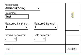
The user has to choose the output file name (as defaults value the project name is recommended), select the measurement lines he wants to evaluate and select the decimal separator and field delimiter. A click on **Accept** starts the export procedure. A bar in the lower part of the window shows the progress.
