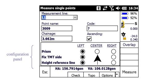
The **Check** soft key starts the control point measurement (Ch. 13.2.2).
