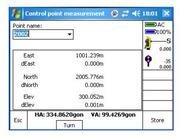
By pressing the **Turn** soft key you can turn the instrument automatically towards a selected reference point.
