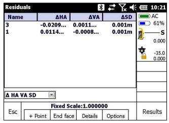
Using + **Point** adds an additional observation to the list of measured points. Therefore the measurement dialog is displayed again. It is not possible to ad an already used reference point to the stationing unless it is previously deleted (see **Details**).
