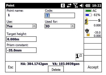
After all measurements are made and the points are activated or deactivated correctly the user may press on **Results** in the **Residuals dialog**.
