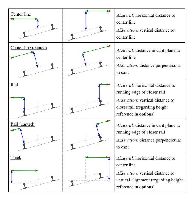
Lateral offsets (shown in graphic as green lines) are defined in ascending chainage direction. A positive value describes a point on the right hand side of reference point (center line or running edge of rail). Points with negative lateral offset are on the left hand side.
