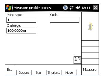
The **Scan** soft key located in the lower center of the screen enables the scan mode. As soon as a reasonable start and end angle were defined the scan will be started by pressing the **Scan** soft key.
