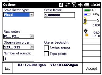
After all settings have been made and the user continues to the next dialog he has to enter the point name of the first target. The point can also be chosen from the reference point list. **Method** defines if the point is measured with or without distance measurement (and therefore may be used only for orientation calculation). Press **Measure** to start the measurement.
