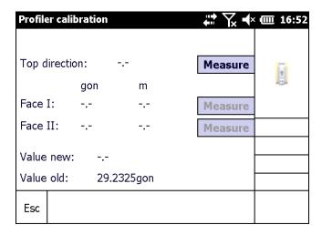
Roughly current orientation of profiler has to be defined after positioning the trolley in the track. Therefore measure with laser at the zenith (straight up, perpendicular to superelevation).
