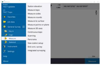
Enter the start point number, code and target height. Make sure the Method shows Angle and distance. Ensure that the correct prism target type is selected using the button on the top menu. Press Measure after locking to the prism target to take each measurement.
