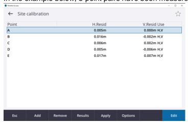
Note after more than 4-point pairs have been measured, both the horizontal and vertical residuals are shown. If a residual is considered too high, after checking the points used, it is possible to tap on the line relating to the point and set its usage to Off, Horizontal only or Vertical only. The residuals for all the points will then recalculate.
