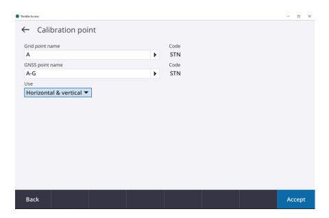
The screen above shows that by default both the Horizontal and vertical coordinate components will be used to compute the site calibration. Later it might be necessary to change this parameter to Off, Horizontal only or Vertical only. Press Accept to return to the Site calibration point table.
