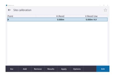
Move to the next calibration point location and press the Add button. Repeat the steps to add a second Grid and GNSS point pair to the calibration. In the example below a second point pair has been measured.
