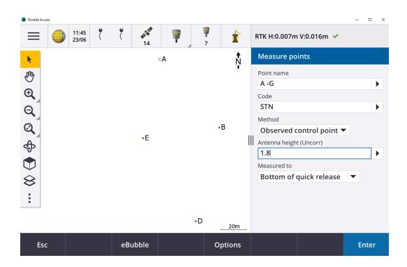
Once the point has been measured, the previous screen will appear showing the name of the Grid and GNSS points.
