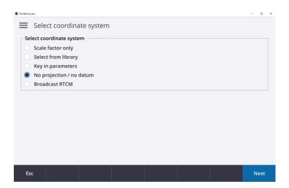
When creating a No projection / no datum coordinate system it is important to specify whether the Local Grid points are provided in Grid or Ground units. If measured with a total station then <u>Ground</u> should be selected.
