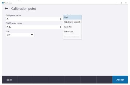
The observation method should be set to Observed control point or Calibration point. Set the Antenna height and measured to position, and carefully measure the calibration point.
