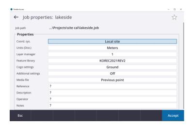
It is a good idea to keep the Site calibration job as a separate job and not use it for surveys or setting out. To transfer a calibration to new jobs, from the Jobs menu – create a new job.
