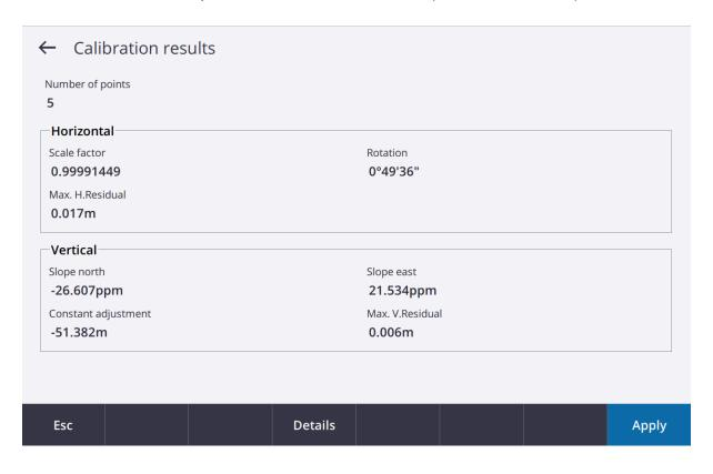
Press **Apply** to apply the results of the calibration as the coordinate system for the job.
