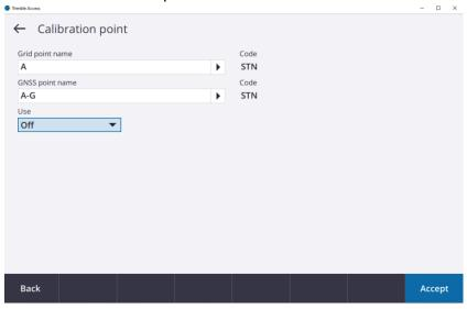
Next enter a name into the GNSS point name box, tap on the right facing arrow and select **Measure**.
