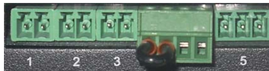
Figure 1-4 User dry contact and opto-coupled connectors
