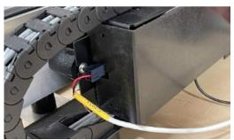
This is a Molex connector and the control cable we include in your kit will have this on the end, so it'll be easy to plug into.
