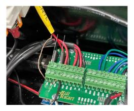
You'll be attaching the PWM cable RED wire into the "PWM" and BLACK into the "GND" pins found along the top-left side of the Mill Right terminal board.
