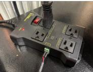
You'll need to supply your own IoT Power Strip as well as a 22awg 2-conductor wire capable of handling up to 5v and <1amp.
