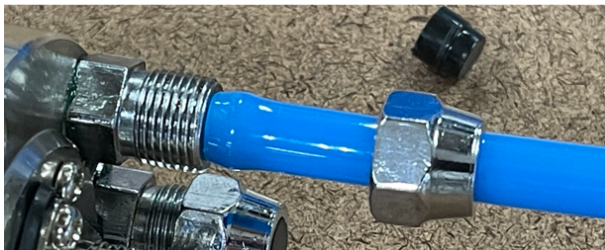
Slip the hose through the nut and onto the nipple.
