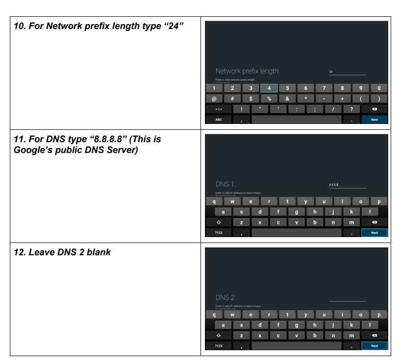
13. After selecting Next, A message should appear at the bottom right of the screen saying "Ethernet connected". (If there is an ethernet cable plugged in.)
