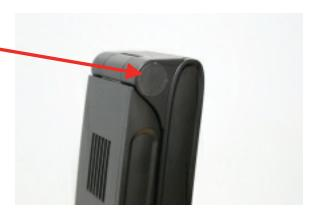
2. Remove the rubber grommet using a flat blunt object.
