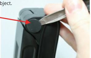
3. Tighten the hinge bolt with an 8 mm or 5/16 inch wrench. Note: You will need to apply more force than expected to turn the bolt. Tighten the bolt about ¼ to ½ of a revolution then test the hinge by opening and closing the camera. Repeat until hinge feels tight enough for proper movement of camera arm.
