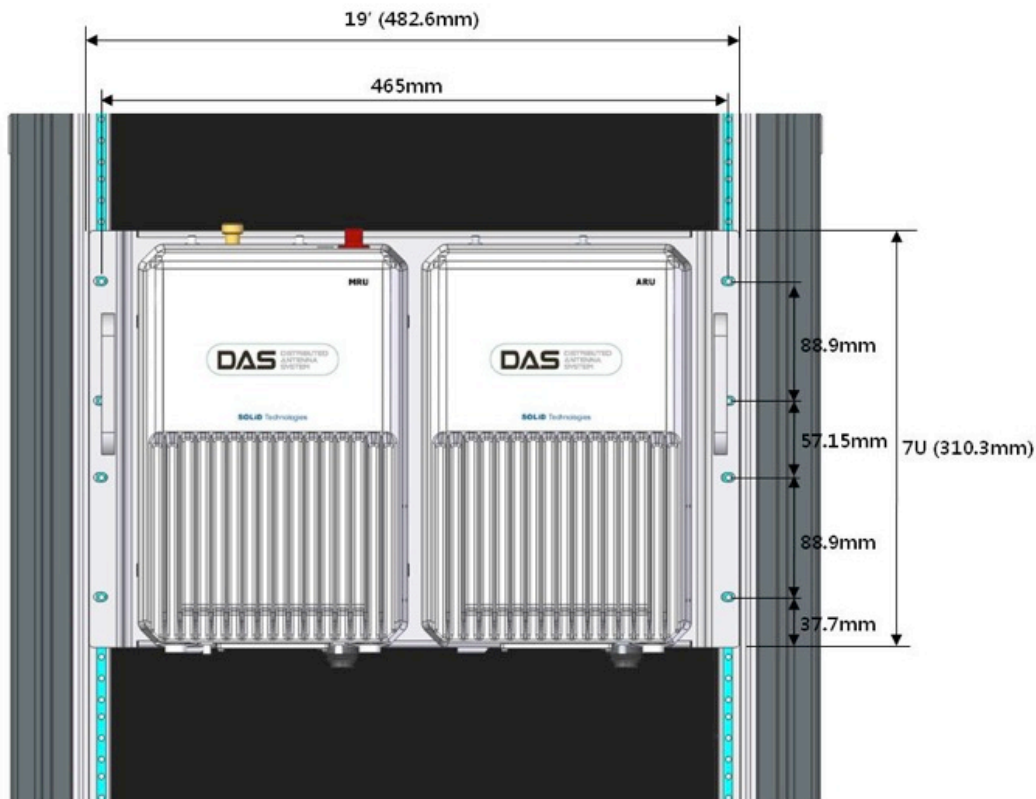
Figure 10.5 – Dimensions for MRU/ARU Vertical Rack Installation
