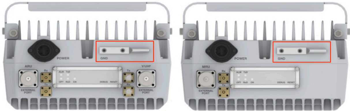
Figure 10.10 – MRU / ARU Ground Terminal
