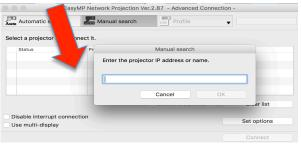
A window will open requesting the IP of the projector. \*You get this info when you press LAN on the projector remote, it displays on the board.
