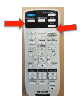
Make sure your projector remote looks like this. You will need to toggle between the LAN & Computer buttons. Select LAN to use the Wi-Fi connect--it will display the \*IP and Keyword you will need to type into the Easy MP Network Projection software on your laptop.
