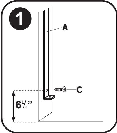
**1.** Install hinge bracket (A) to wall (stationary side of gate) using Phillips screw (C) beginning 6 1/2" above floor surface.
