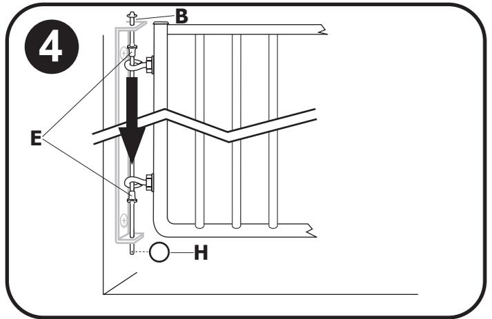
**4.** Hang gate by inserting hinge rod (B), through top of mounted hinge bracket (A), through upper plastic shoulder washer (E), through both eye bolts, through lower plastic shoulder washer (E), and finally through bottom of hinge bracket. To secure hinge rod, insert key ring (H) through hole in end of hinge rod.
