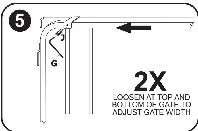
**5.** Set gate to width by holding latch assembly against mounting wall (see beginning of **STEP 6**). Use Allen wrench (F) to insert set screws (J) and tighten top and bottom of gate.
