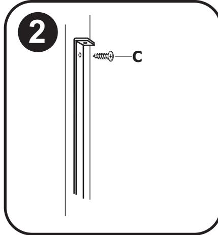
**2.** Install second screw (C) in top of hinge bracket securing it to the wall.
