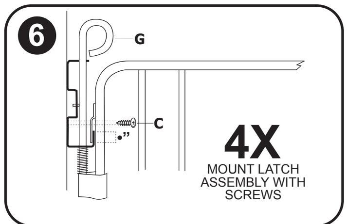
**6.** Hold latch assembly (G) against opposite wall and extend gate until at least 1/2" of safety bracket will interlock with flange of latch. Mark position of latch assembly screw holes with pencil. Swing gate out of way and mount latch assembly to wall. Check closure of gate and tighten set screws from STEP 5 to secure gate width.
