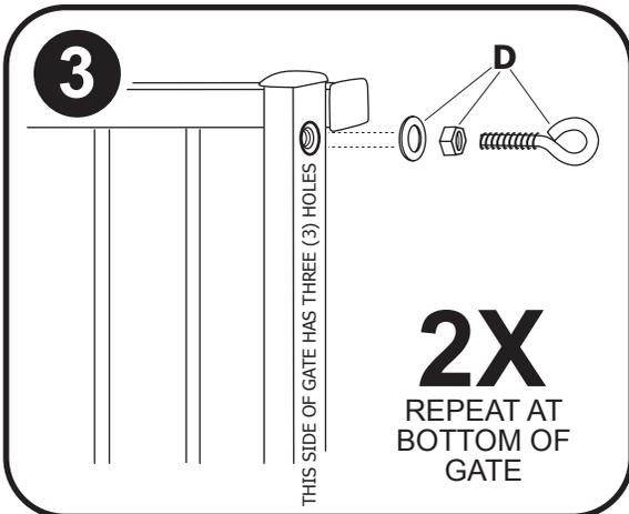
**3.** Insert eye bolts (D) into top and bottom of hinge side gate (side with three holes). Be sure nuts are tight.
