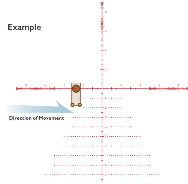
2.74 mrad correction for a target moving at 3 mph at 800 yards. No wind. Total bullet time of flight from trigger pull is 1.5 seconds during which the target travels 6.6 feet. Elevation already dialed into turret.
