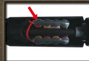
Insert the battery into lower handguard then reinstall upper handguard.
