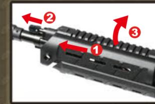
Push the upper handguard forward and pull the knob toward flash hinder then pull out upward.
