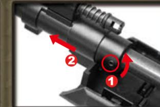
Unscrew both side and take off the front barrel.
