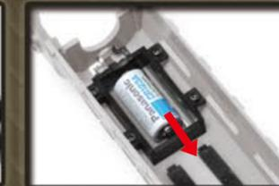
Pull out the cover and insert the CR123A battery.
